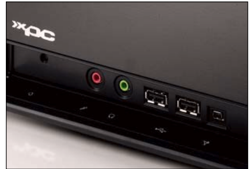
USB, Firewire and audio ports are accessible via a flap at the front
